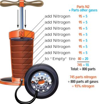
When you take an "empty" tire and add enough 95 percent pure nitrogen to bring its pressure up to about 105 psi, the nitrogen concentration inside ends up being about 93 percent.
