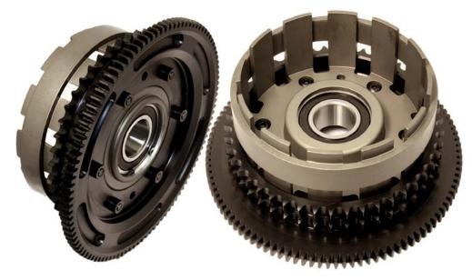
Evolution Industries 46 And 49 Tooth Billet 6061 Hard Anodized Aluminum 2 Piece Clutch Basket With Steel Sprocket And Ring Gear, The 49 Tooth Gear Raises RPM To Achieve Maximum Performance Eliminating Lugging Of Motor.
